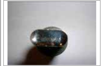
Punch tip edges are easily damaged, usually from poor handling practices, rarely from operation.
