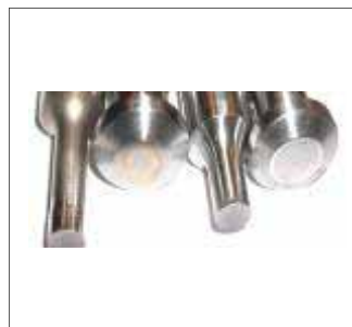
Double Impressions are caused by punches twisting and jumping during compression
