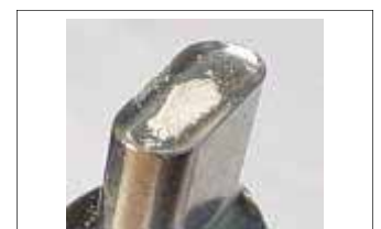
Sticking occurs when particles adhere to the punch face
