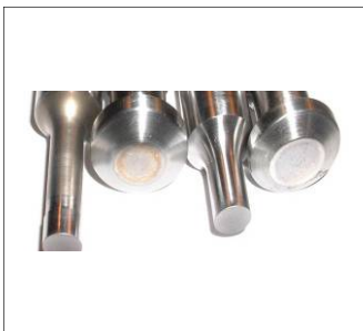
Double Impressions are caused by punches twisting and jumping
